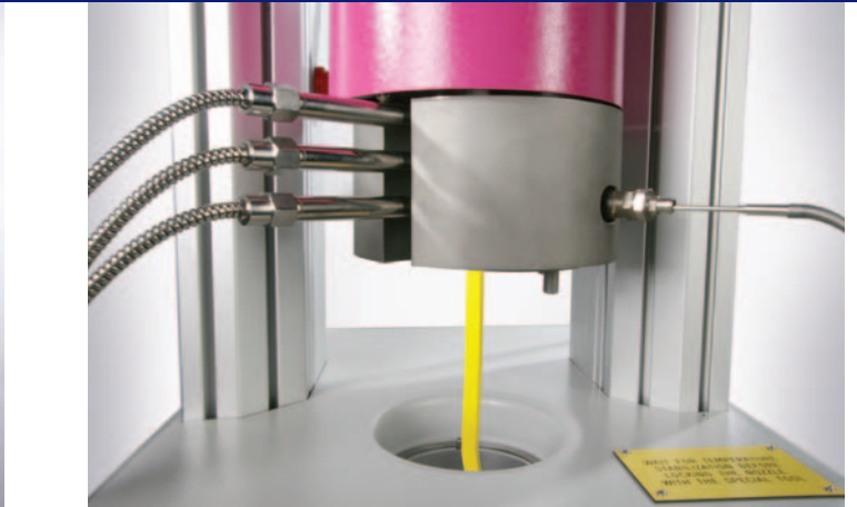
Detail of Slit-Die system
